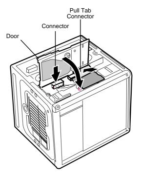
5 Close the AirPort shield door, and press it down so the door latch engages.
